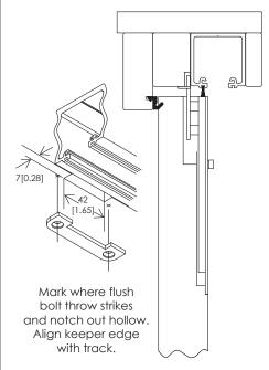
Install 456 '1' Type Channel Flush Bolt for bottom (only available in 1 size)
