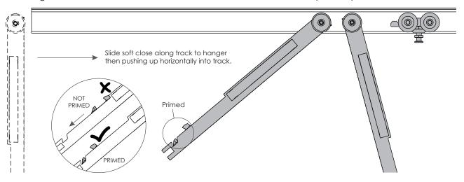
Insert 2nd hanger & attach hanger to soft closes with cap screws. Install panel as per system instructions.
