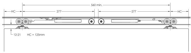
Zero Clearance 60 (min panel width 610mm)
