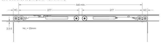
Cavity Clearance 60 (min panel width 700mm)
