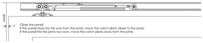
Adjust catch plate as required. Secure in final position with the 3rd screw
