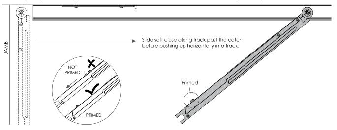
Insert 2nd hanger & attach to soft close with cap screw. Install panel as per system instructions.
