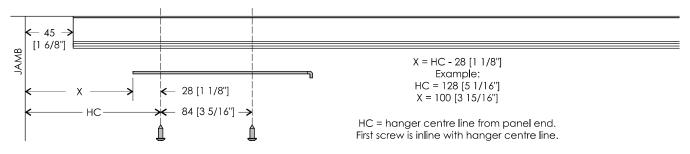
Insert clip stop &1st hanger into track, then soft close. The soft close must be in primed position, as shown
