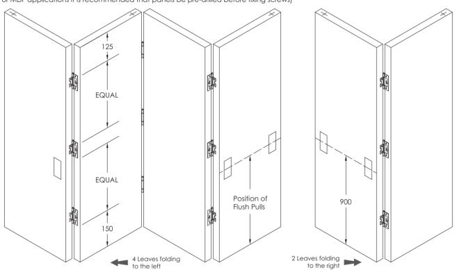
Position flush pulls as shown in positions shown in Hardware Orientation on page 4. If door knobs are preferred, they need not be fitted until the end. Note - on a 5½ or 6 leave unit, door knobs cannot be fitted on the middle leaves. Flush pulls are recommended for these applications. Sold separately.
