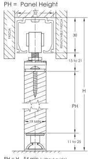
PH = H - 54 min (without guide) PH = H - 59 min (with guide)
