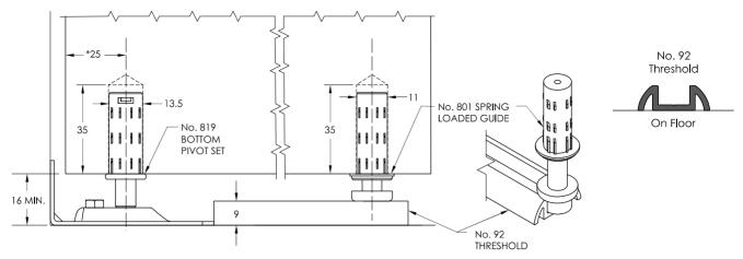
Butt threshold hard up against wall bracket. On units with door width less than 22mm \*25 must be 28mm.
